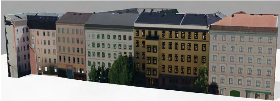
Figure 9: A virtual street scene in LoD3 built by enhancing LoD2 models using our proposed pipeline.
