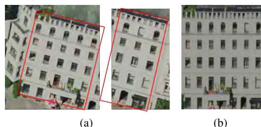
Figure 2: (a) An example in which a wall consists of two raw texture images taken from non-frontal views. We combine the areas enclosed by the red boxes together to form one piece of wall texture image. (b) The generated wall texture image for this example.
