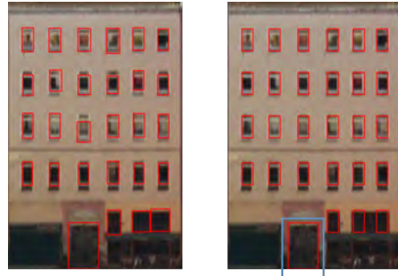
Figure 4: The sub-figures on the left and right show an example of the original facade element detection result and the result after adjustment, respectively. In this example, N_{cluster} = 3 .
